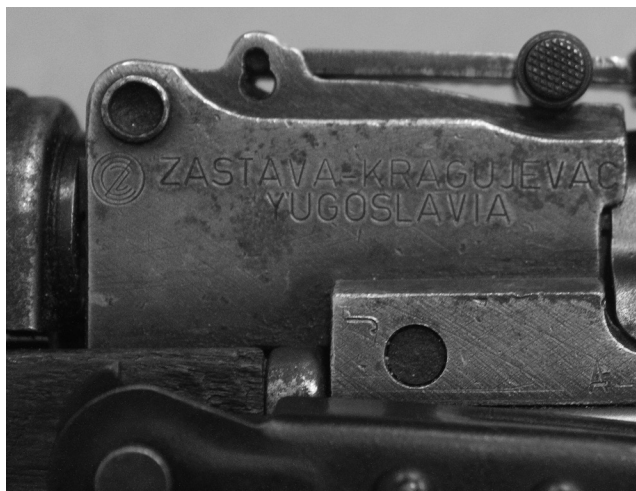
Figure 4.61 This image is a close-up showing the markings on the left side of an AK barrel trunnion. In this case, the manufacturer is Zastava, located in Kragujevac, Yugoslavia (now Serbia). This marking dates the manufacture of this AK to prior to the breakup of Yugoslavia. Many Eastern Bloc AKs were marked on the barrel trunnion, and not necessarily on the receiver itself due to space considerations. Many thousands of Zastava AKs were demilled and sold as “parts kits” to the U.S. market, allowing builders to install these on a new receiver. The receiver must be researched for markings, as these other markings would be erroneous for identification. (Image from author’s collection.)
